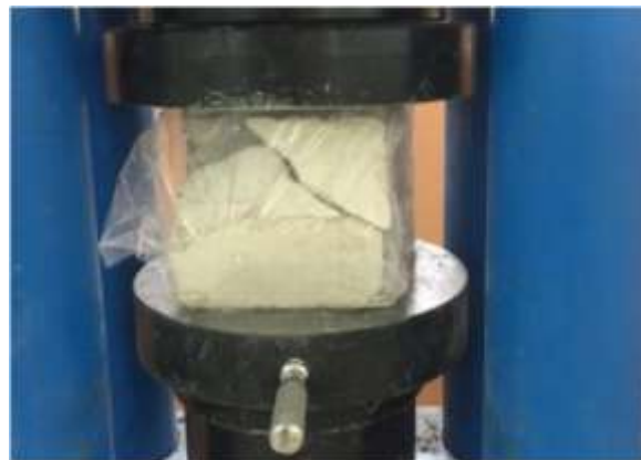
Fig. 3. Initial crushing of source cubes.
