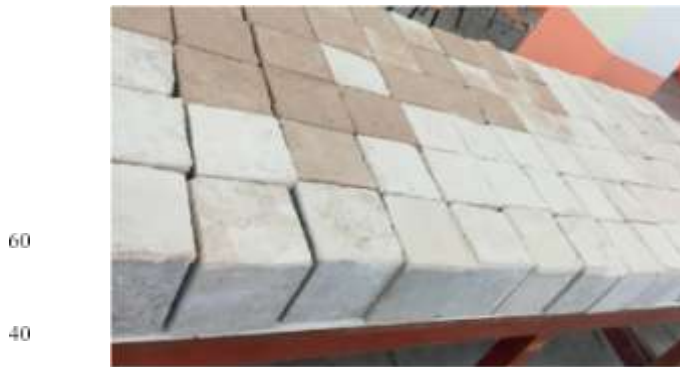
Fig. 2. A batch of source gypsum-plastered cubes.
